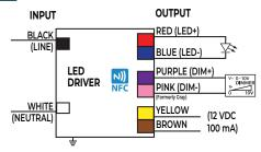
Note: Gray (-) dimming wire has been changed to pink per the 2020 NEC section 410.69 and NEMA.
