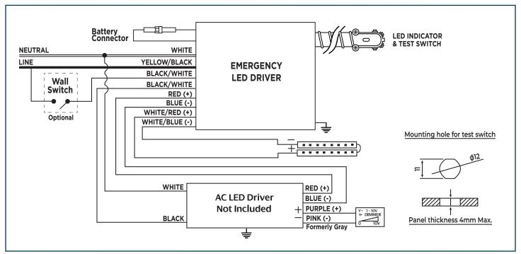
Maximum wiring distance: 18 feet using 18 AWG wire.
