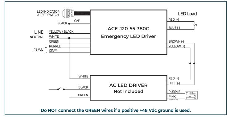
If a delay is needed for the AC LED DRIVER when transferring back from emergency-mode to normal-mode when normal power is restored, then connect the BLACK wire from the AC LED DRIVER to the BLACK wire of the Emergency LED Driver directly or through the WALL SWITCH if used.
