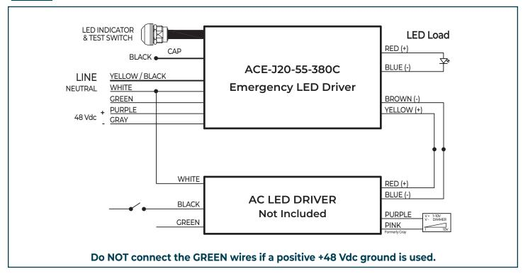
If a delay is needed for the AC LED DRIVER when transferring back from emergency-mode to normal-mode when normal power is restored, then connect the BLACK wire from the AC LED DRIVER to the BLACK wire of the Emergency LED Driver directly or through the WALL SWITCH if used.
