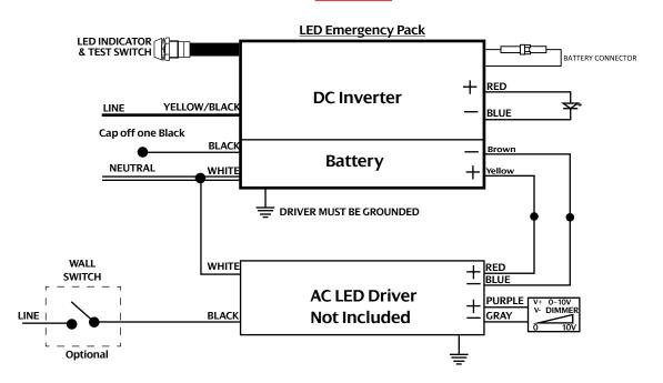
Input Voltage: 120-347V, 50.60Hz • Surge Rating 3Kv
