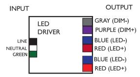
Both output postive and negative connectors are equivalent (same eletrical point)
